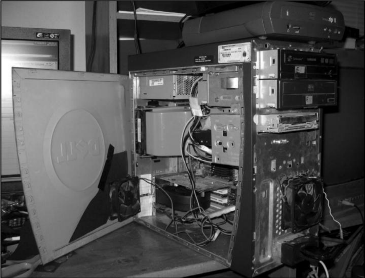
Figura 02.4: Retirando as tampas do gabinete.
